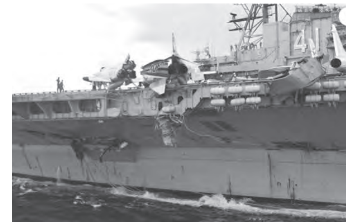
The Cactus struck near the carrier's liquid oxygen plant, killing two sailors working in the plant and injuring three others.
